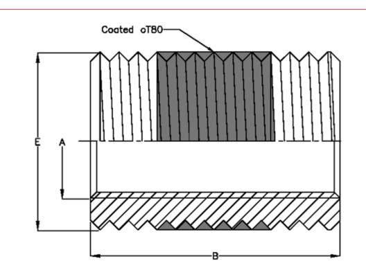
Female thread A = M10Length B= 20Male thread E= M14Type= 97x 000 100.100
